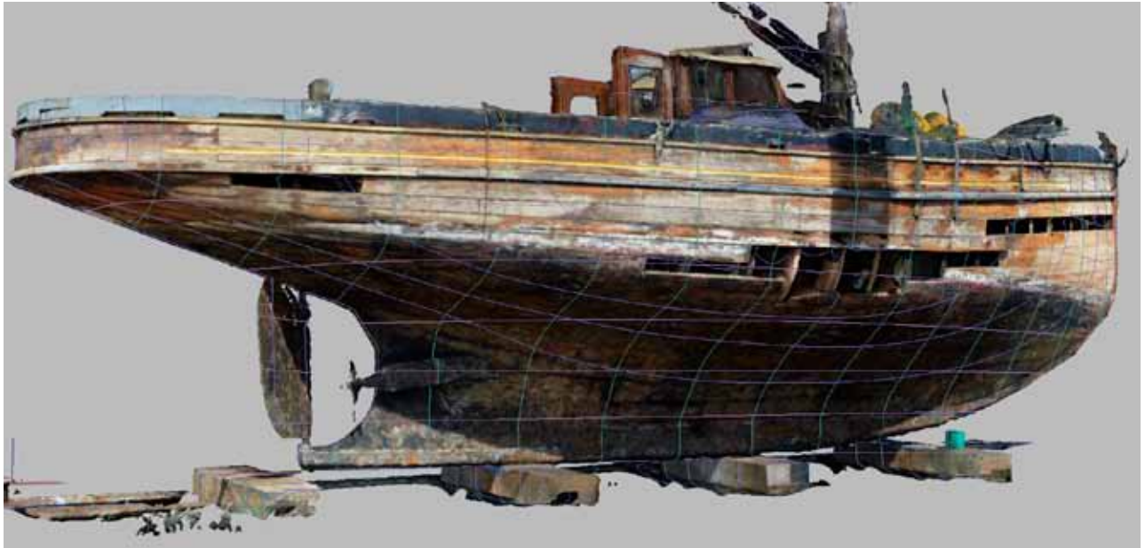
Above & Below: Photogrammetry renderings from bow and stern views used to accurately re-create the lines of the nobby Aileen.
